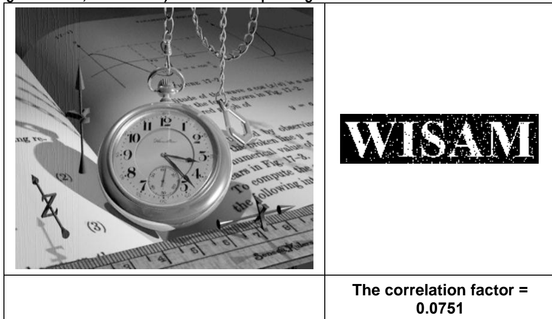
Figure 4.40: The attacked watermarked image “Clock” using 'Image Glow' (radius=1, brightness= 10, contrast=10) with its corresponding extracted watermark
