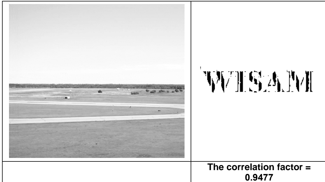
Figure 4.39: The attacked watermarked image “Field” using 'Image Glow' (radius=1, brightness= 10, contrast=10) with its corresponding extracted watermark
